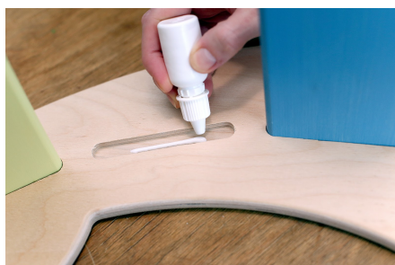
6. Put glue in the empty sockets
