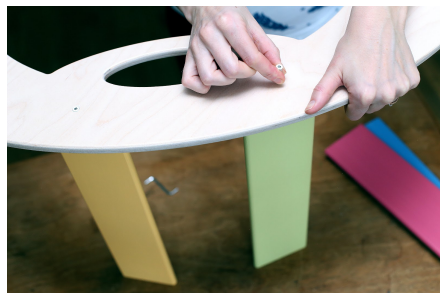
4. Put the rest 3 laths in the sockets
