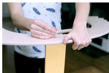
2. Put the first lath in the socket
